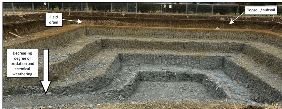
Figure 4. Example observational trial pit (Oxford Clay, (OxC) at surface).
