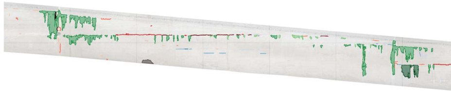
Figure 5. Example of orthomosaic image and identified defects at Block 41.
