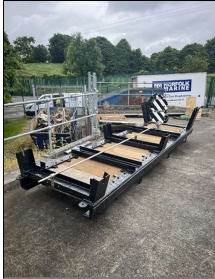
Figure 8: Renovated Limpet Cofferdam On-site Ready for Installation
