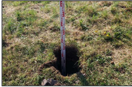
Figure 11 : Modified soakaway hand dug pit at Lower Foulridge.
