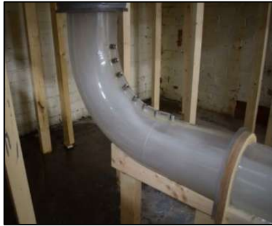
Figure 5. Existing spillway physical model (90-degree bend)
