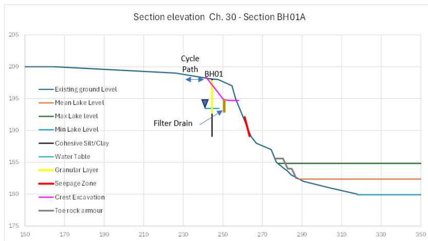
Figure 10. Original depth of filter drain which had to be subsequently raised to avoid tufa seepage zone
