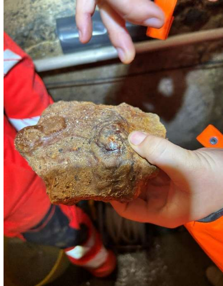
Figure 10. Example of hardened mineral deposits removed during the cleaning exercise
