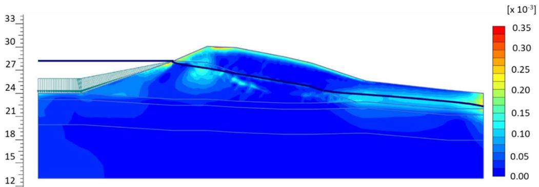
Figure 7. PLAXIS output showing shear strain after 10 years (end of Summer).
