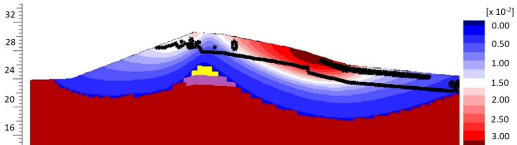
Figure 6. FLAC output showing total displacements (metres) after 10 years with material boundaries in background as per Figure 3 and phreatic surface shown in black.
