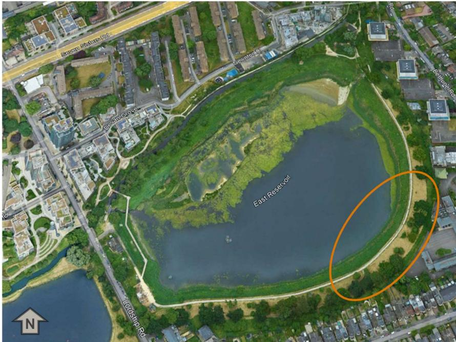
**Figure 1.** Stoke East Newington Reservoir with area of highest settlement circled © Google (2024).
