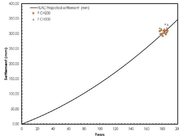
**Figure 11.** Retroactive projected settlement of FE analysis vs normalized predictions from settlement monitoring at CH200 and CH300 (normalised to 2010).
