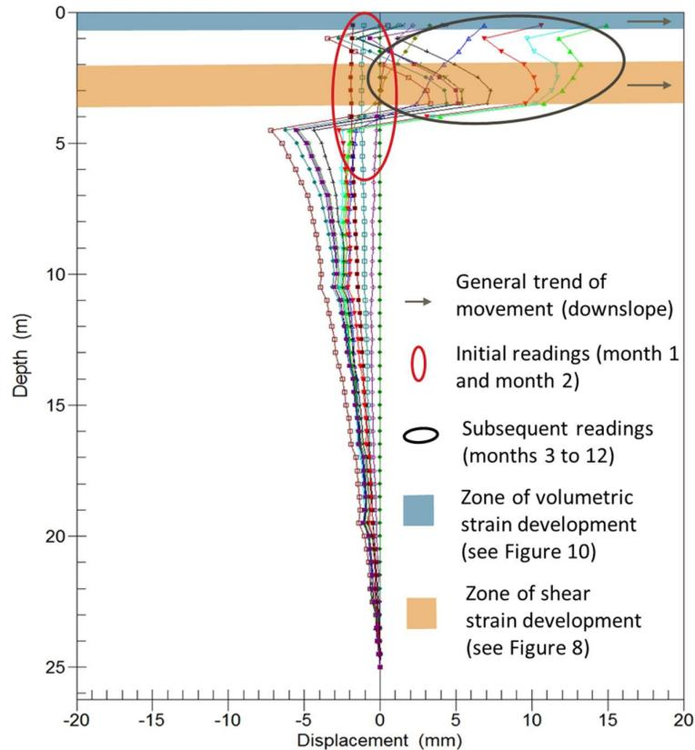
Figure 9. Cumulative inclinometer results between initial installation on 2<sup>nd</sup> July 2020 and 23<sup>rd</sup> June 2021 for the embankment section under investigation.
