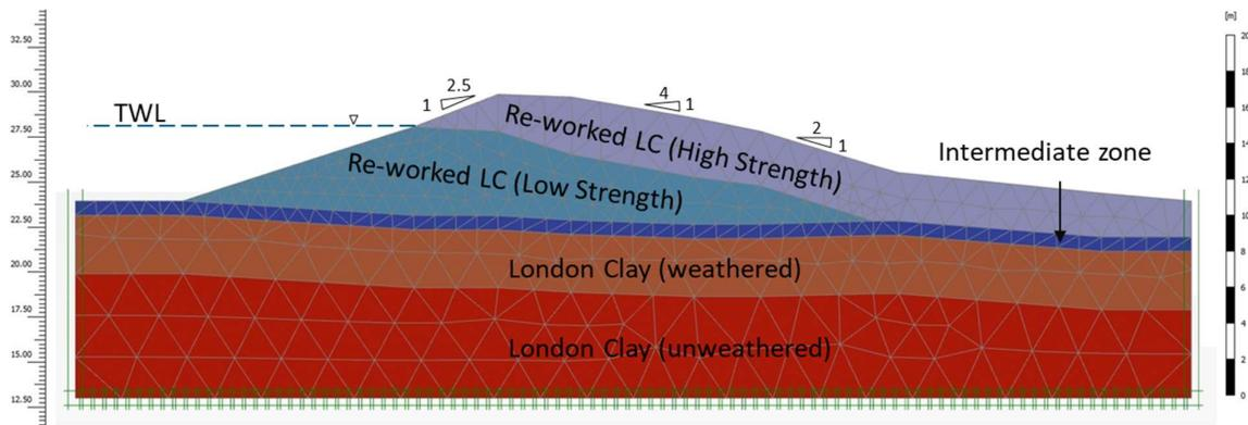
**Figure 3.** Cross section at CH 273 analysed in PLAXIS and FLAC.
