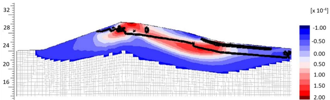
Figure 8. FLAC output showing shear strain after 10 years and phreatic surface shown in black.
