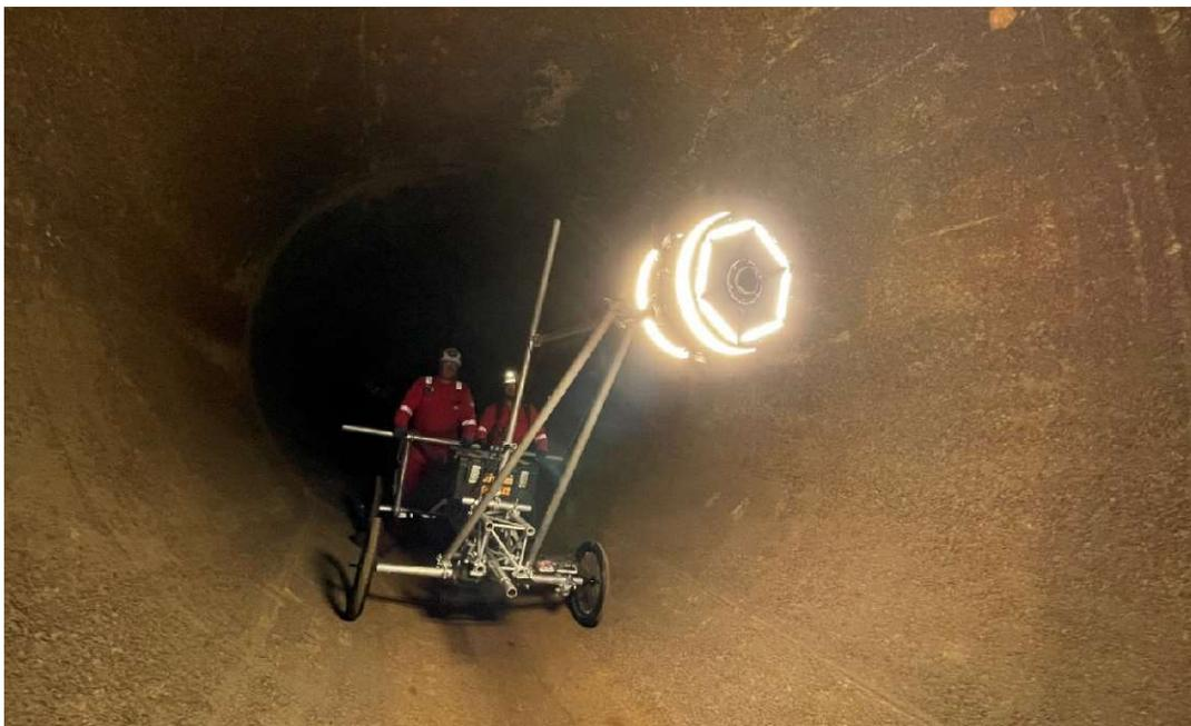
**Figure 4.** Tunnel Inspection Vehicle, implementation in c.4m diameter configuration
