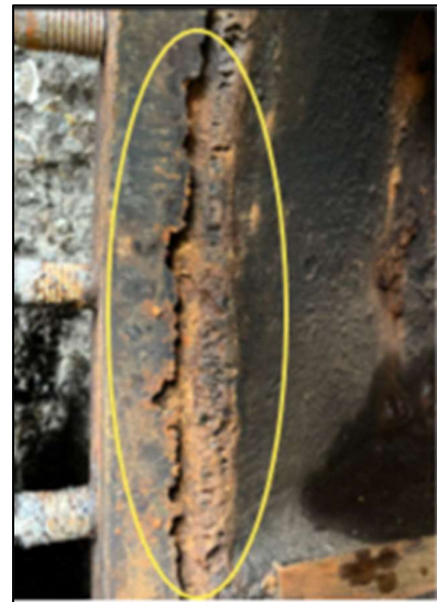
Figure 7. Cavitation to valve body
