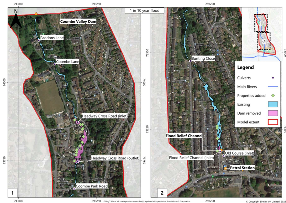
Figure 10. Example change in flood outline by removing the dam – 1 in 10 year flood
