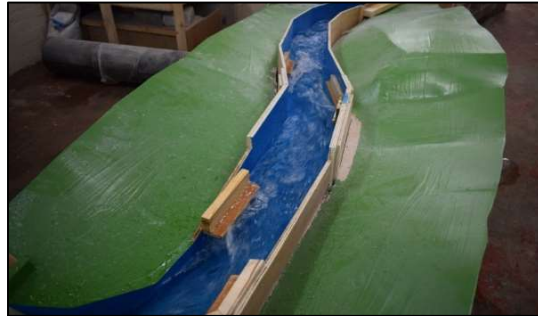
Figure 13. New spillway layout at 44\text{m}^3/\text{s} (as modelled)
