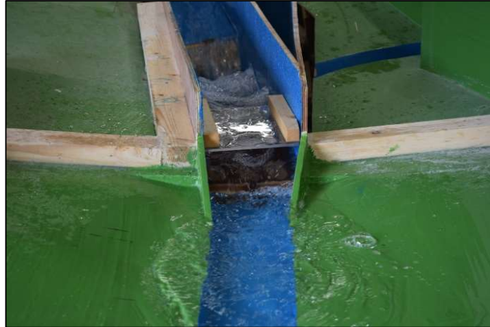
Figure 14. Stilling basin in 1 in 150-year flood event (as modelled, looking upstream)
