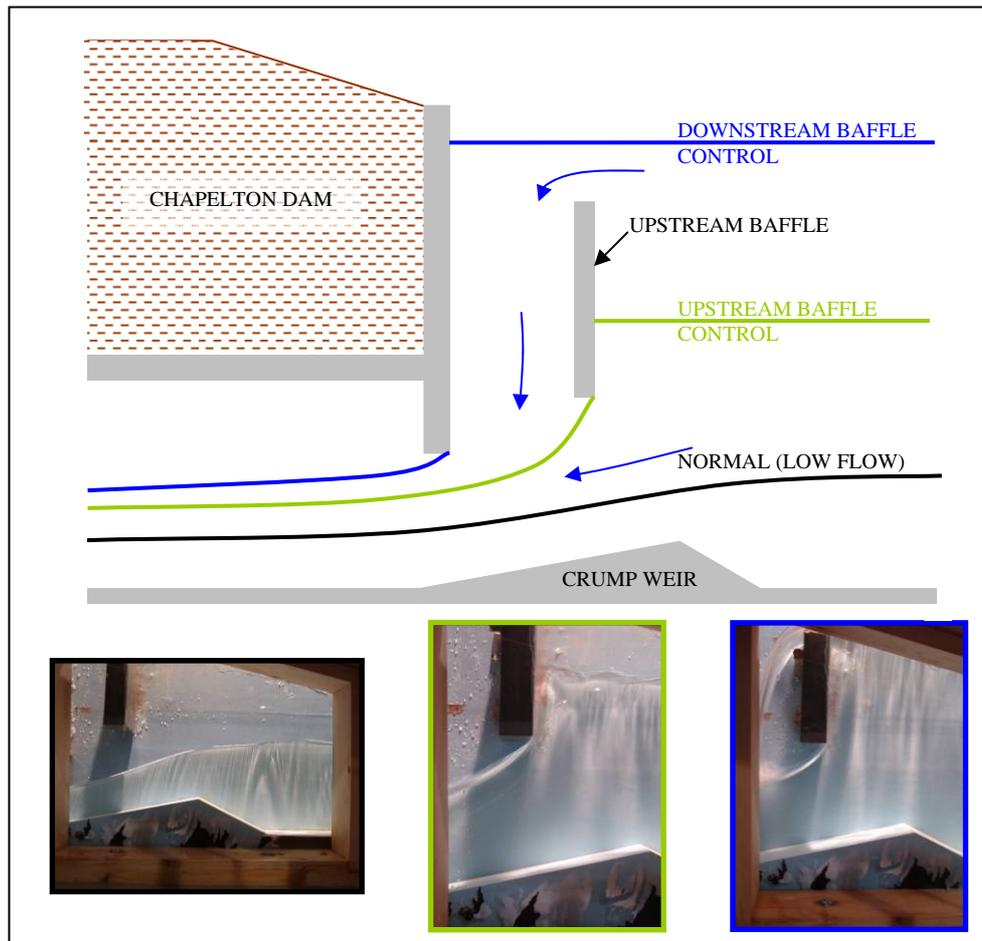
Figure 3. Baffled crump weir concept
