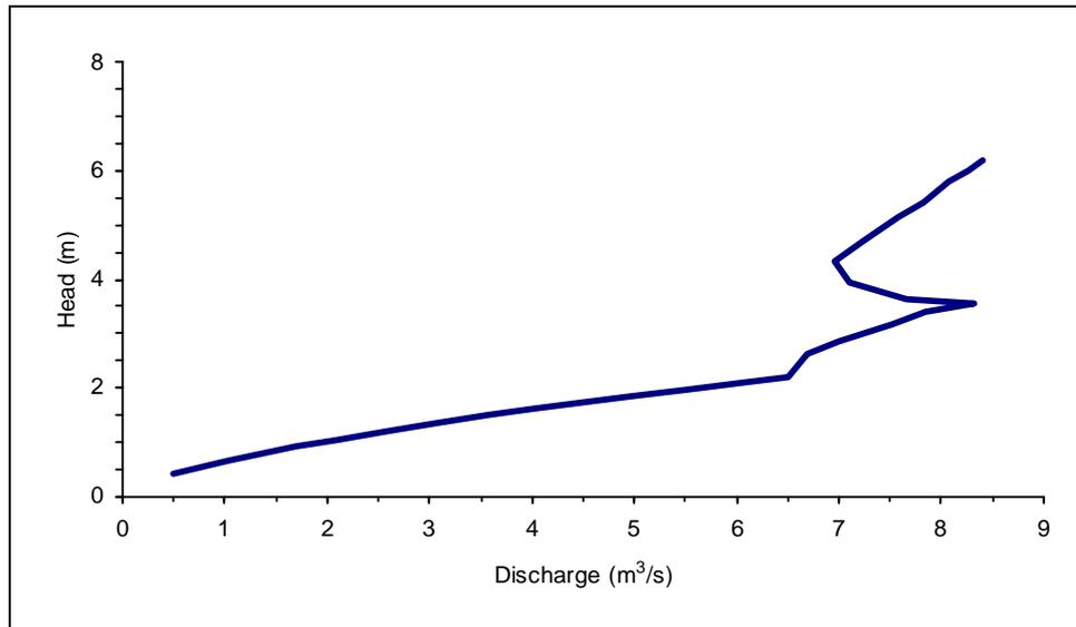
Figure 6 Baffled crump weir stage vs. discharge
