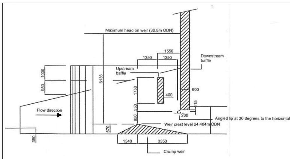
Figure 5. Optimised arrangement
