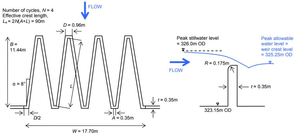
Figure 5. Labyrinth weir dimensions
