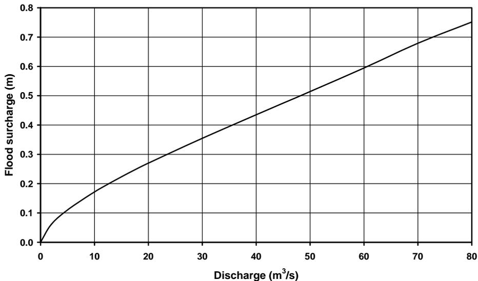
Figure 6. Rating curve for Craig-y-Pistyll labyrinth overflow weir
