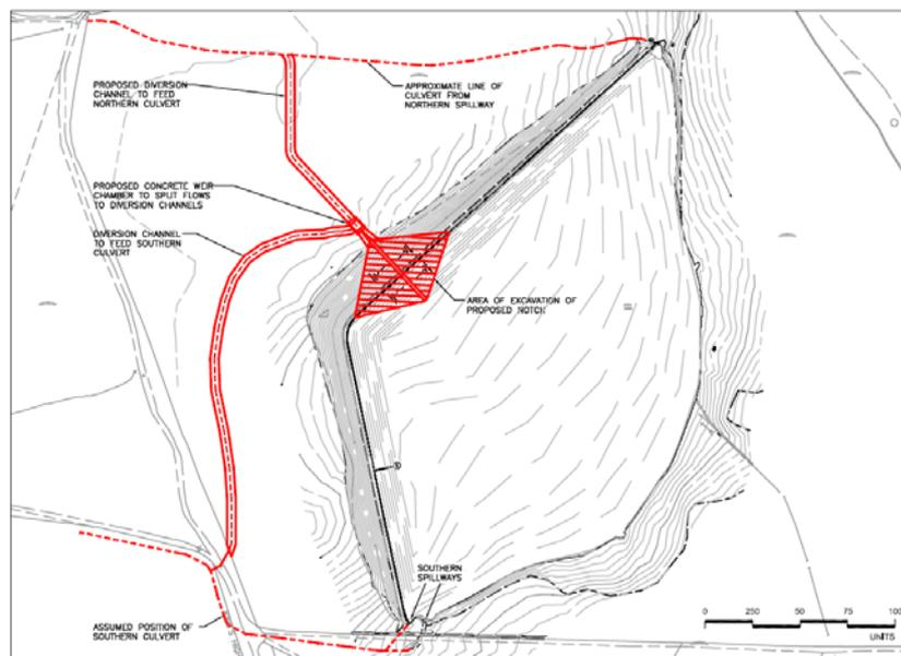
Figure 2. General Arrangement of Preferred Option in study (2a) (full height notch with diversion channels to north and south culverts)
