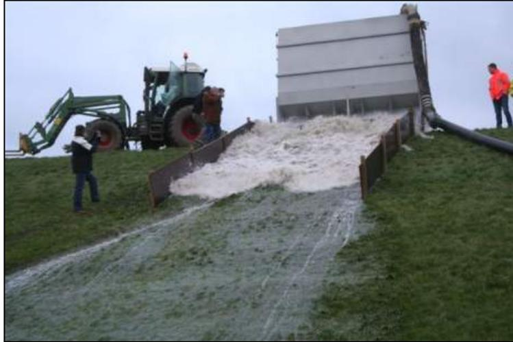
Figure 6. Wave overtopping simulator in action on a dike in The Netherlands
