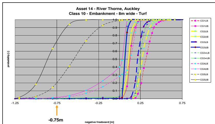
Figure 5. The fragility curve for the breach at Auckley suggested a very low probability of failure at 0.75m below crest when failure actually occurred
