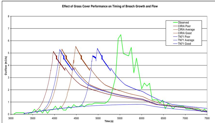
Figure 1. Comparison of breach outflow predictions against observed test data using CIRIA 116 grass performance curves and original TN71 performance data.
