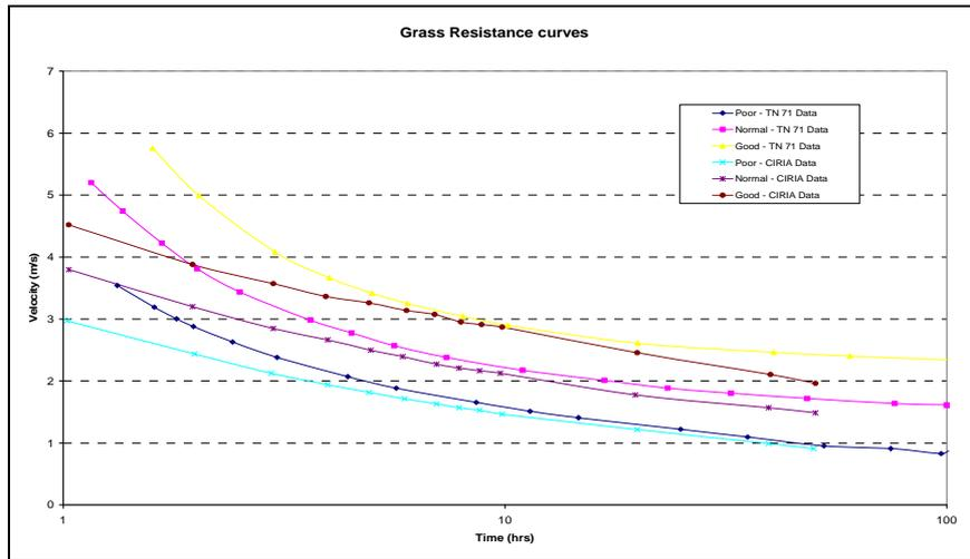
Figure 2. Comparison between CIRIA 116 (Hewlett et al., 1987) performance curves and the original TN71 field test data (Whitehead et al., 1976)
