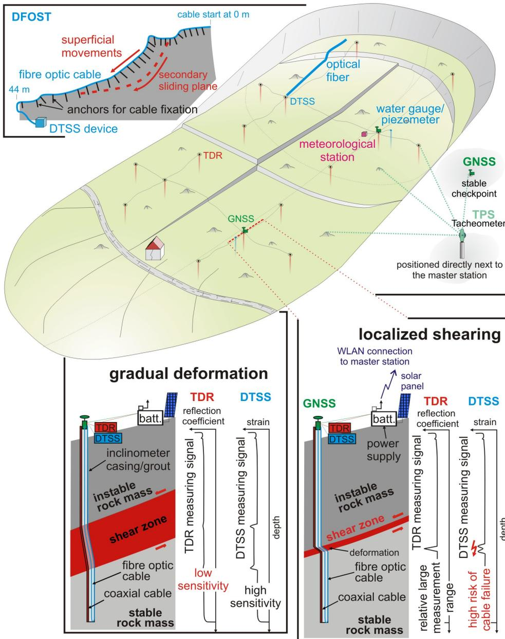
Figure 3: Measuring setup and expected measurement data at the Aggenalm Landslide.
