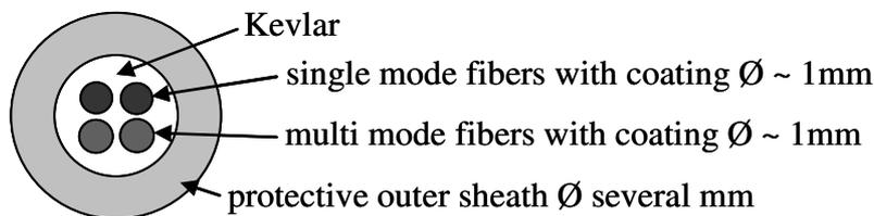
Figure 1: Cross section of a strain sensing cable.
