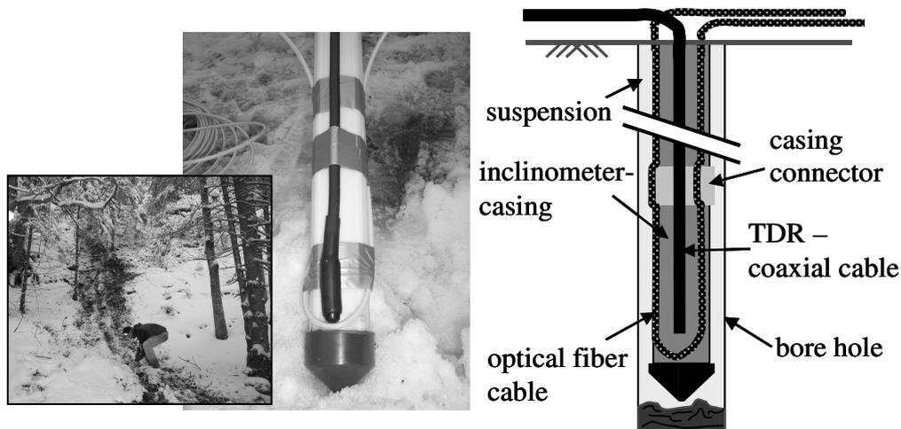
Figure 2: Equipment in the vertical borehole: TDR cable, optical cable and inclinometer and near-to-surface cable installation during snow fall (left)
