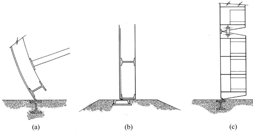
Figure 4. Unsuitable arrangement of structural stiffening members at the bottom section of gates
