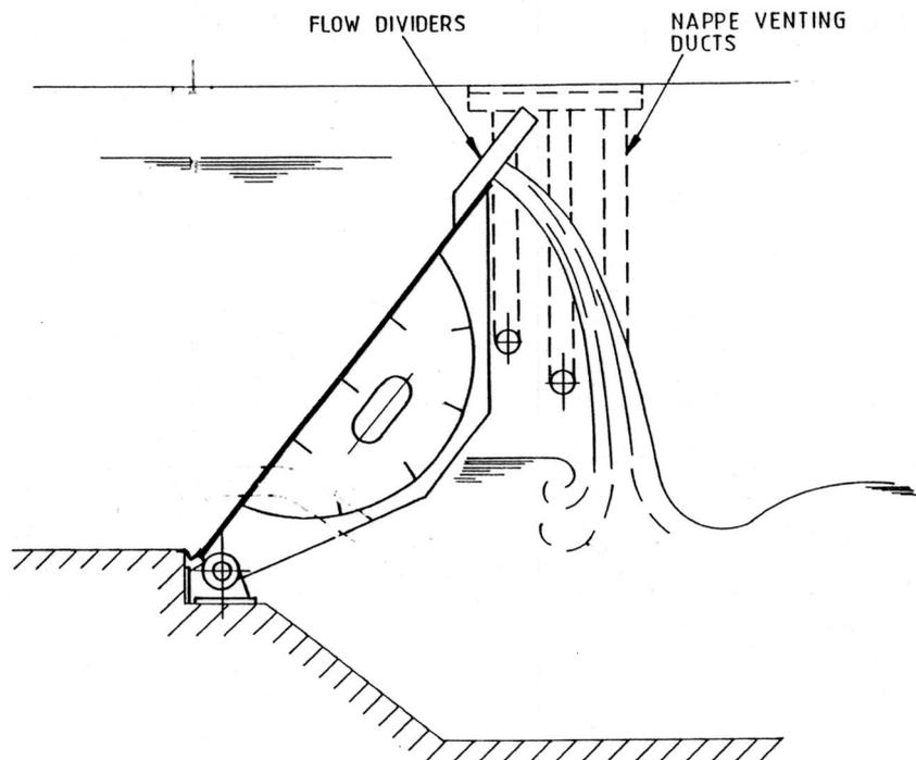
Figure 8. Venting the overflow of a gate
