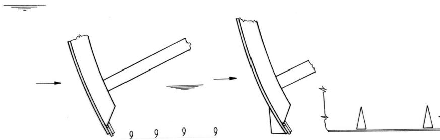
Figure 6. Regular eddy shedding at the bottom of radial gate
