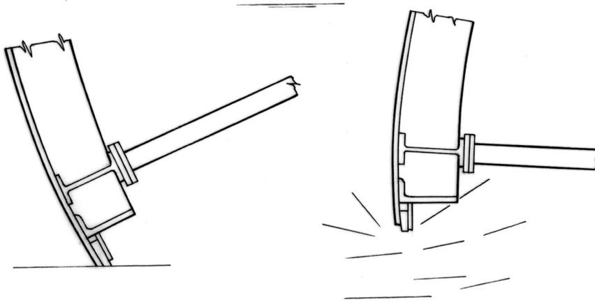
Figure 5. Structural reinforcement of the bottom of a radial gate which can cause flow reattachment when the gate is raised
