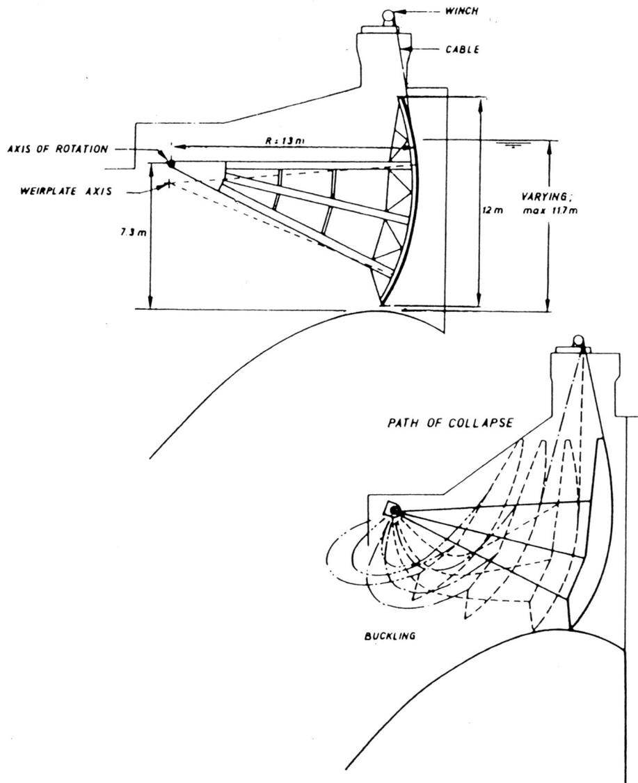
Figure 7. Spillway gate vibrations leading to the collapse of a gate (after Ishii et al)
