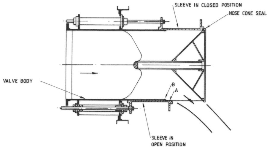
Figure 10. Hollow cone valve
