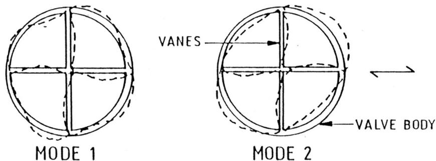
Figure 11. Possible vibration modes of hollow cone valves (after Mercer)
