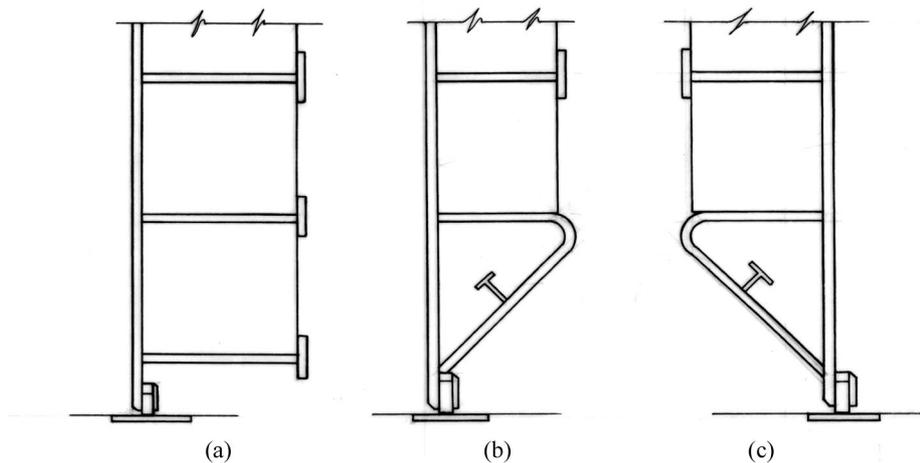
Figure 3. Structural reinforcement of gate bottoms
