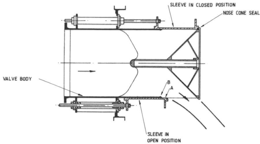
Figure 10. Hollow cone valve
