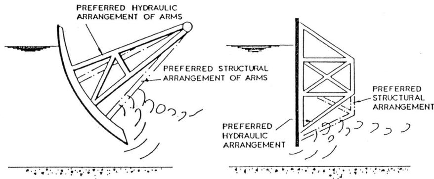
Figure 9. Preferred hydraulic structural arrangement of a gate subject to drowned discharge
