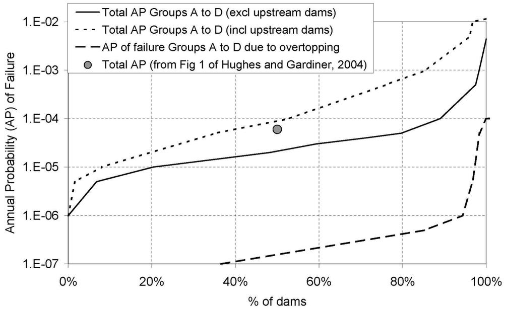
Figure 4: Cumulative distribution of annual probability of failure
