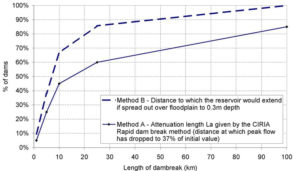
Figure 6: Group E: Alternative methods of estimating length of dam break impact
