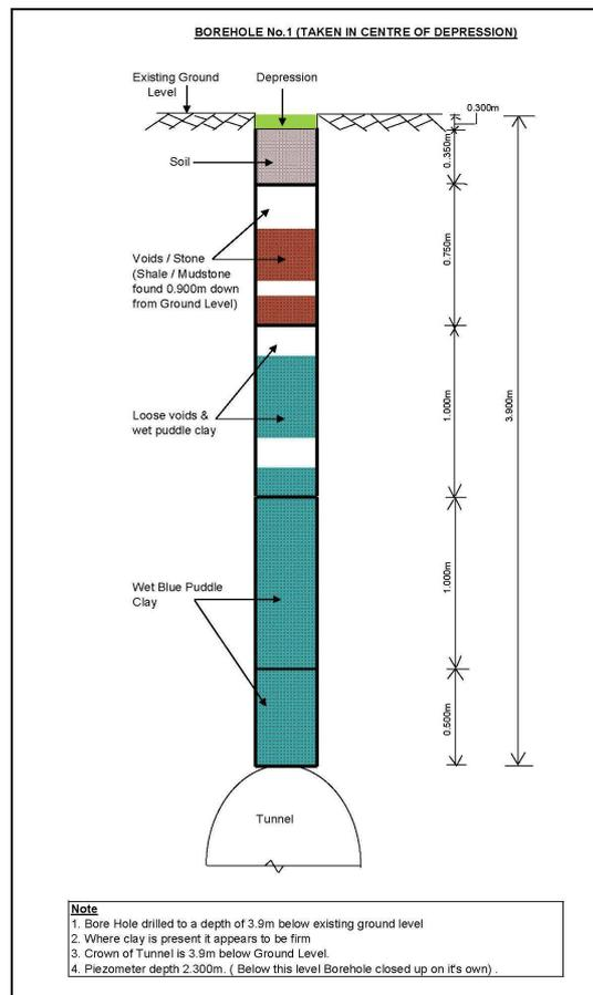
Figure 4 – Schematic log of borehole BH1 in the depression on the crest
