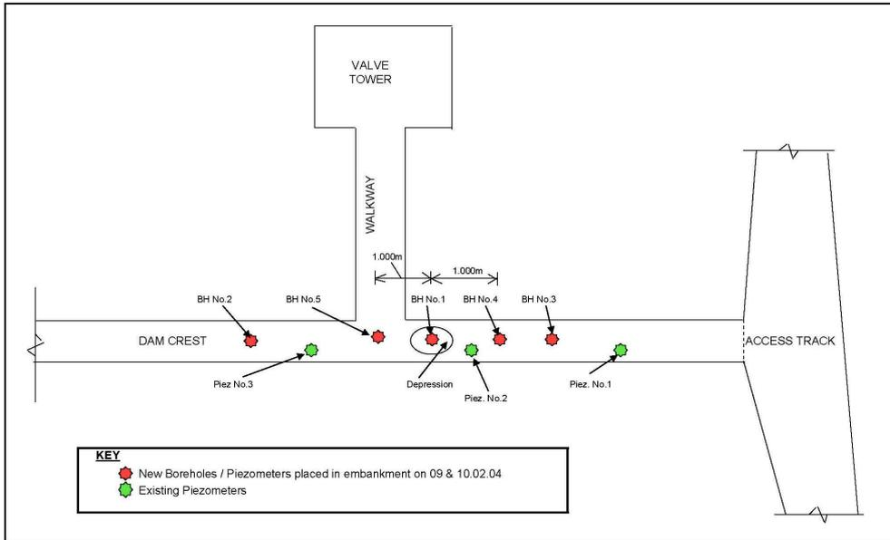
Figure 3 – Plan of Llyn Morwinion - Location of boreholes and piezometers placed in 2001
