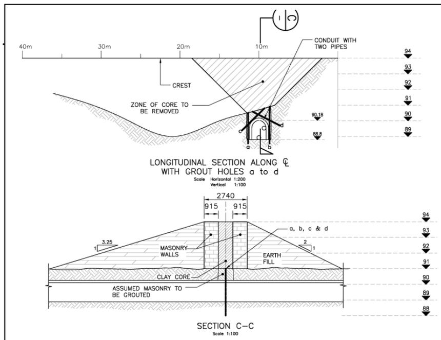
Figure 9 – Longitudinal Section and Embankment Cross-section identifying approximate location and alignments of proposed grout boreholes “a” to “d”
