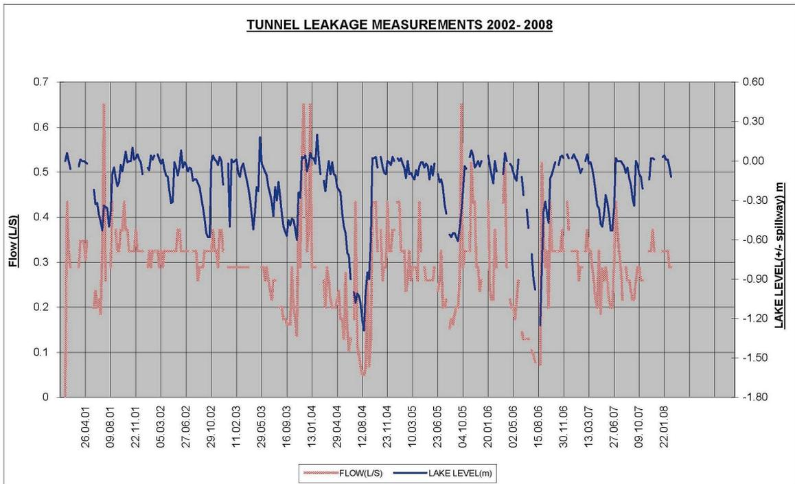
Figure 2 – Leakage into the Outlet Conduit from 2001
