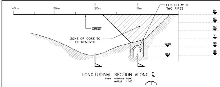
Figure 1 – Longitudinal section identifying hard horizon & conduit
