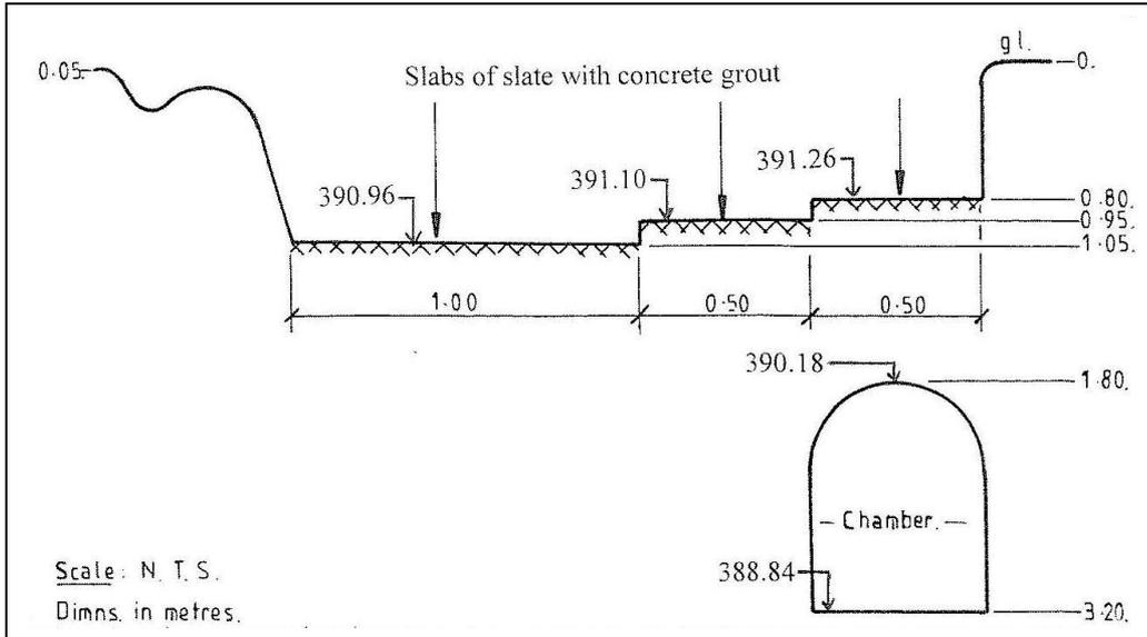
Figure 8 – Log of Trial Pit Downstream of the Embankment
