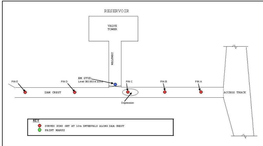
Figure 5 – Location of survey pins placed in the crest in 2001
