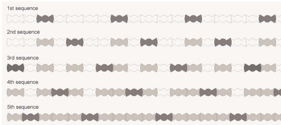
Figure 6: Procedure of jet grouting in five sequences
