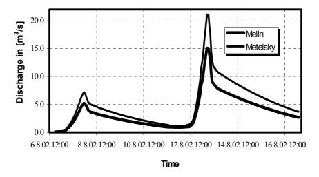
Figure 6: Derived flood hydrograph in August 2002 at the dam sites
