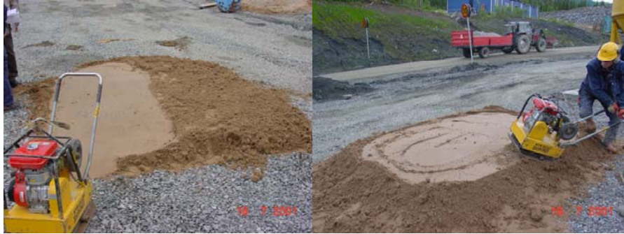
Figure 6. Field trials with BES. At left the trial surface is compacted in layers of 0.1 m and to the right the material is compacted in two layers of each 0.3 m at water content of 15 %.
