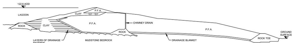
Figure 1: Cross section of the embankment
