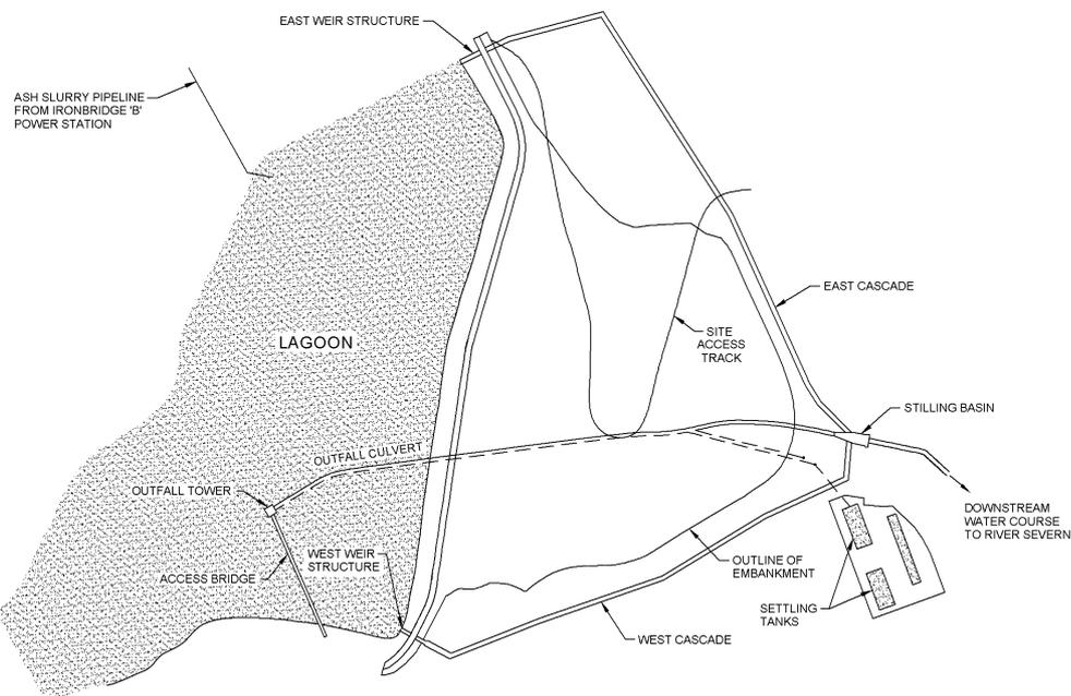
Figure 2: Plan of the embankment at Devils Dingle
