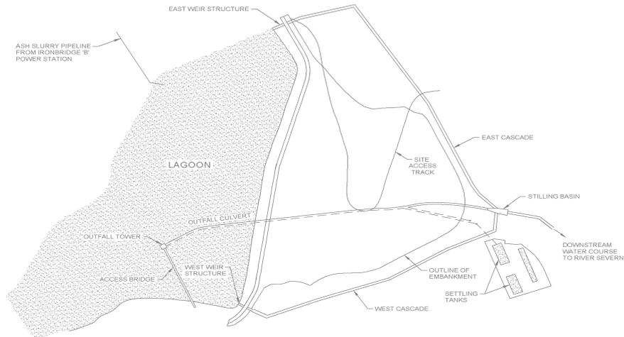
Figure 2: Plan of the embankment at Devils Dingle
