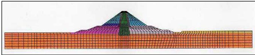
Figure 6. The F.E. mesh for dynamic analyses
