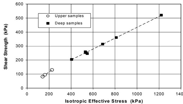
Figure 11. Shear strength vs. isotropic effective stress
