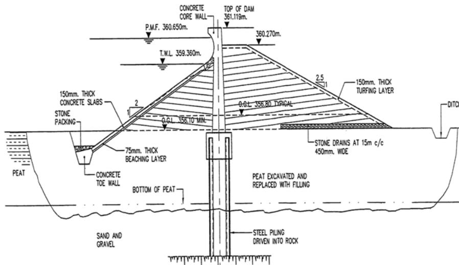
Figure 2 Typical cross section of Dalwhinnie Dam
