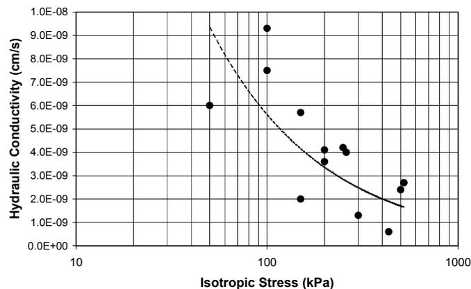
Figure 13. Hydraulic conductivity vs. the isotropic stress
