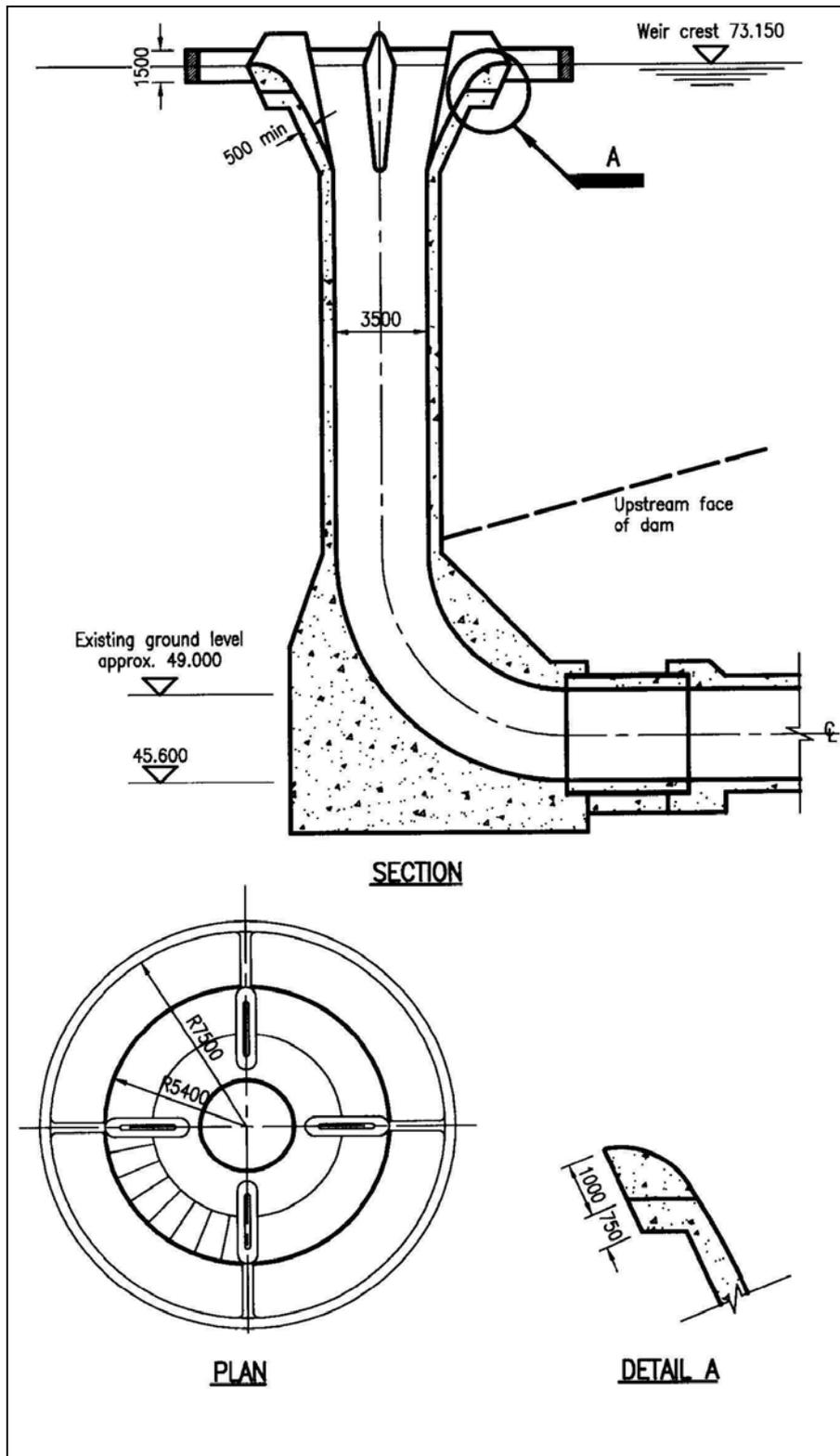
Figure 1 - Detail of the Overflow Structure
