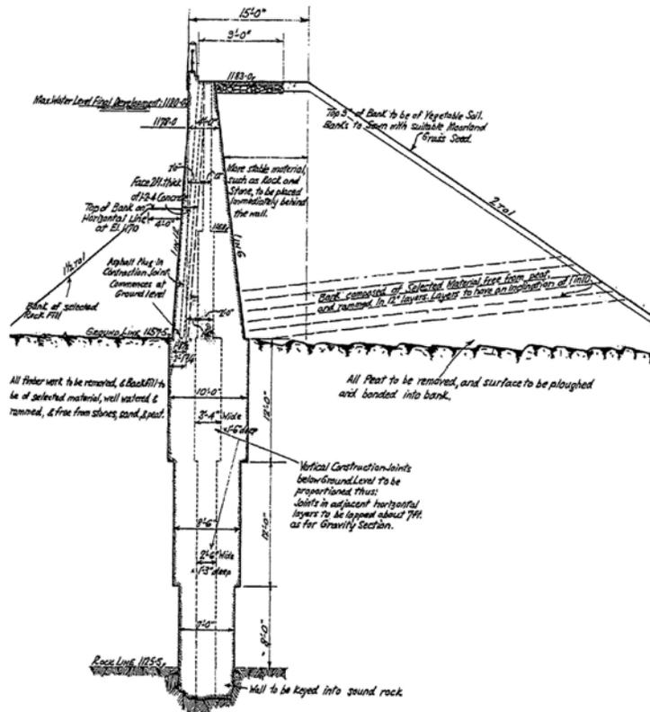
Figure 1 Typical cross section through Ericht corewall Dam
