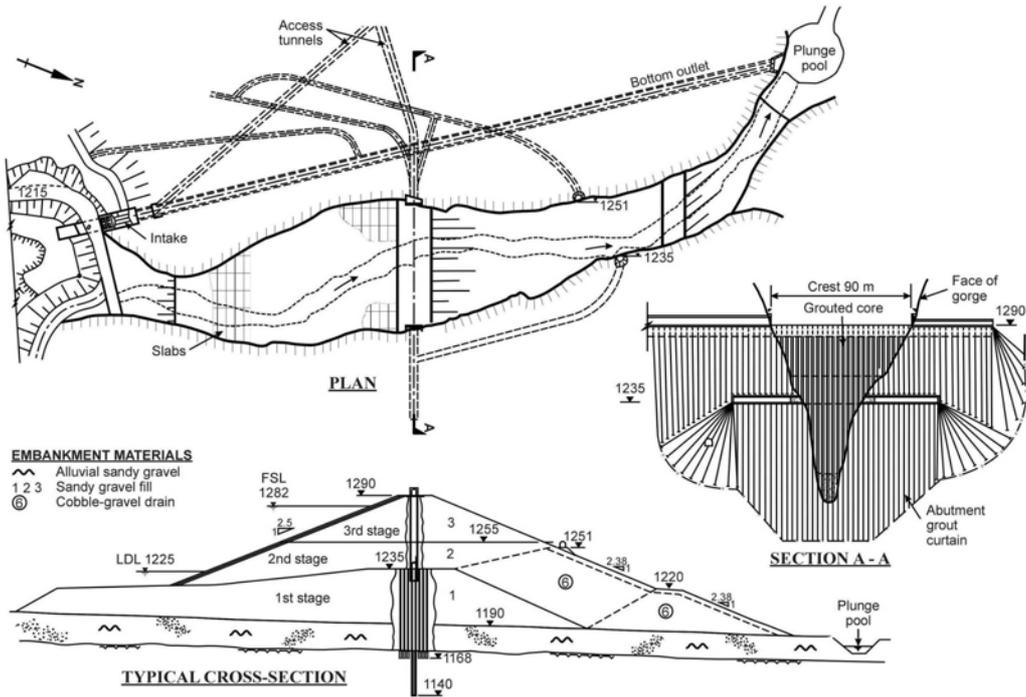
Figure 1. Papan Dam Plan and Sections
