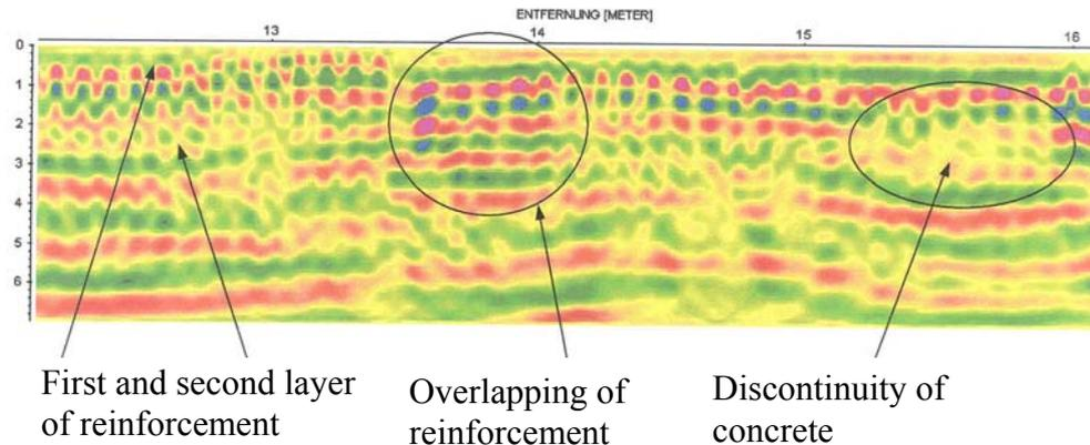
Figure 5: Example of evaluation of Georadar investigation
