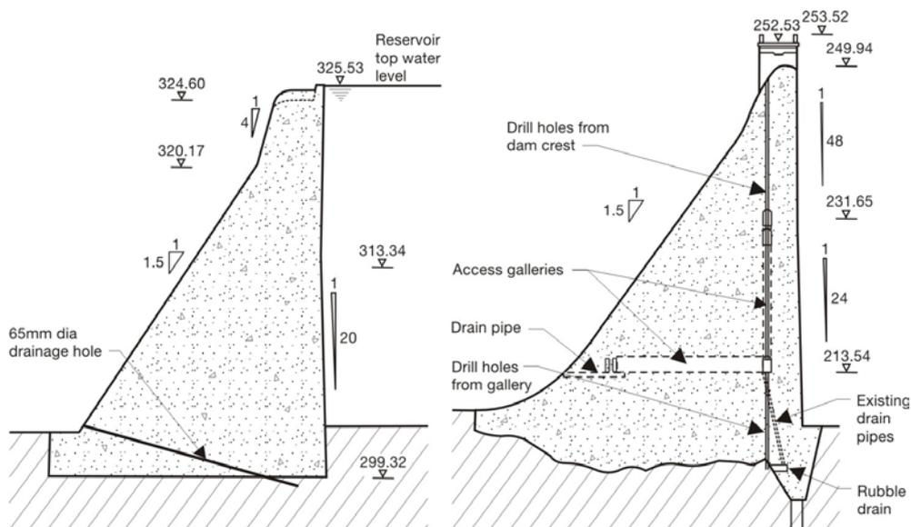
Figure 1 Sections of Blackwater and Laggan dams (not to scale)
