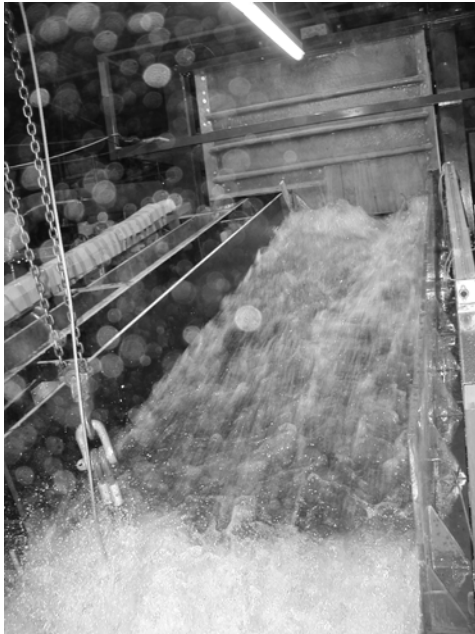
Fig 4: Tilting flume – Self supporting Open Stone Asphalt revetment under a load of q = 360 \text{ l/(sm)} at a slope of 1: 5
