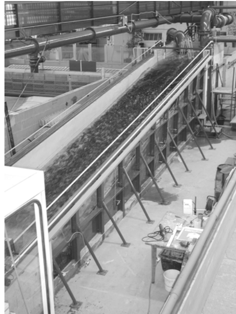
Fig 5: Half dam model for overtopping tests at a slope of 1 : 6 during operation
