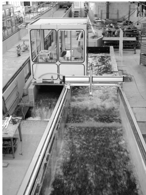
Figure 6: Energy dissipation at the toe of the slope – View from upstream (cf. Bieberstein et al. 2002)
