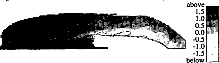
Fig. 10: Hydraulic head distribution for case without bridge (in m)
