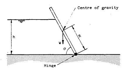
Figure 2: Basic cross section of tipping gate
