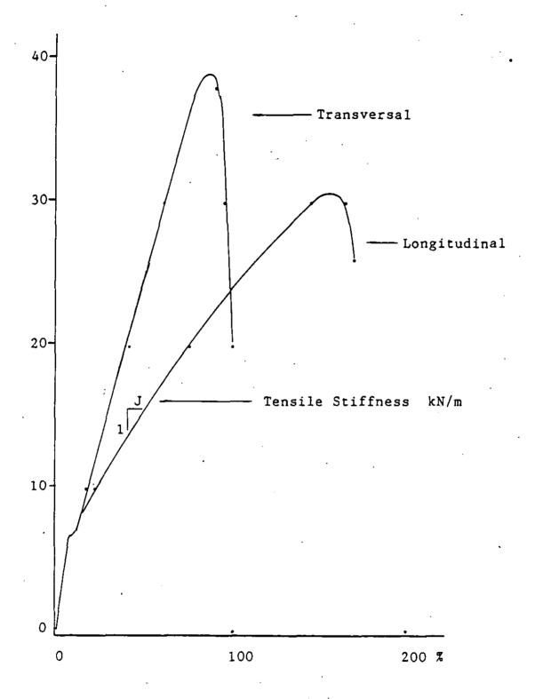
Fig. 1. Tensile Force (kN/m) - Elongation (%) test results of
