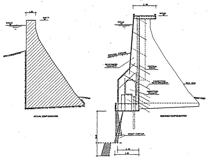
Figure 9: Typical sections of the Tres dams: actual and designed configurations
