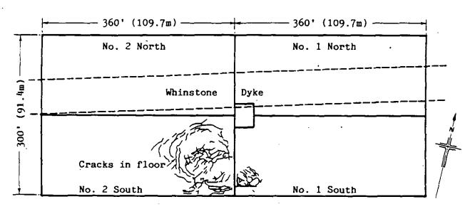
Figure 1: Plan showing cracks in floor
