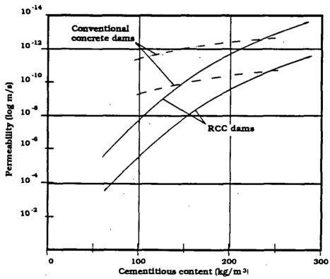
Figure 4: Comparison between the in-situ permeabilities of concretes from RCC structures and conventional concrete dams
