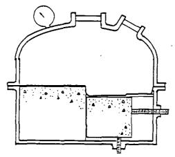
Fig. 2 Pressure chamber modified for stretch and shear tests and definition of parameters measured.
