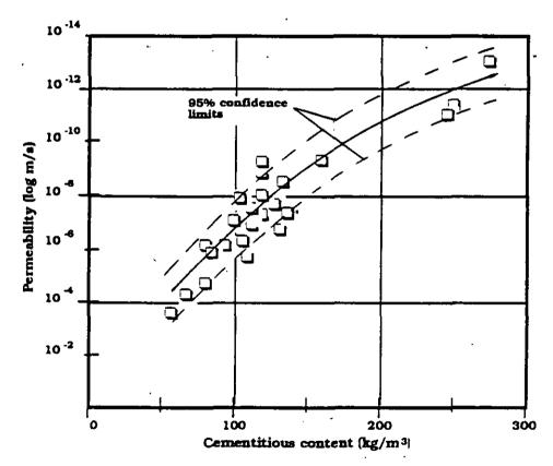
Figure 2: Relationship between in-situ permeability and cementitious content for concretes from RCC structures
