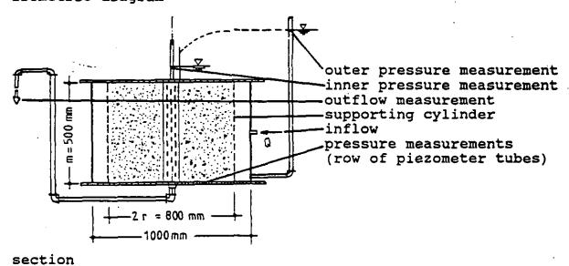
Figure 1: diagram of pressure pot
