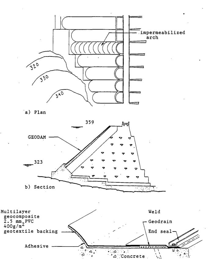
Fig. 5 Concrete multiple thin shell dam repaired with a surface multilayer PVC geocomposite fixed with adhesives.
