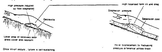
Fig. 3: Failure scenario, geotextile Fig. 4: Failure scenario, concrete reinforced channels block model
