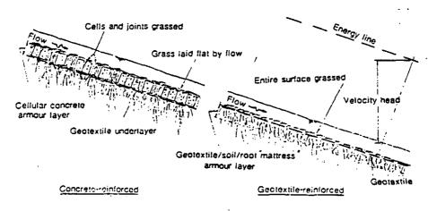
Fig. 1: Cross-section through typical reinforced-grass waterways
