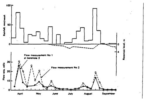
Figure 3: Records of rainfall, reservoir level and flow rate from wet areas at Gorpley dam
