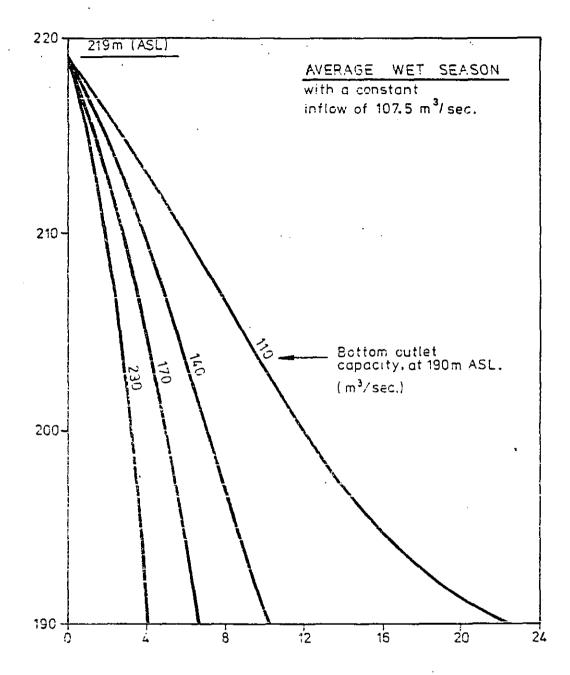
The figure shows graphically the above drawdown times for an average wet season and it is clear that a worthwhile improvement is achieved as the outlet capacity (at a water level of 190m ASL) is increased from  $110\text{m}^3/\text{sec}$  to  $140\text{m}^3/\text{sec}$ . After this improvements are more modest.
