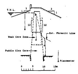
Figure 8: Pore Pressures at Maximum
