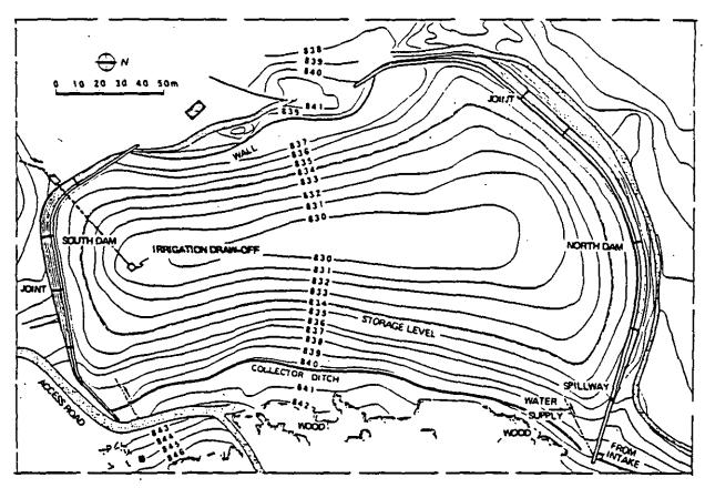
Figure 7: Lay-out of the Tres reservoir: actual situation
