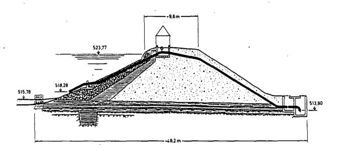
Figure 5: Cross section of Prinzen Dam with new syphon
