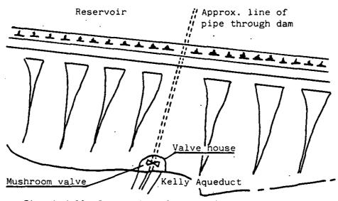
Fig. 1 Kelly Reservoir. Layout of Original Pipework
