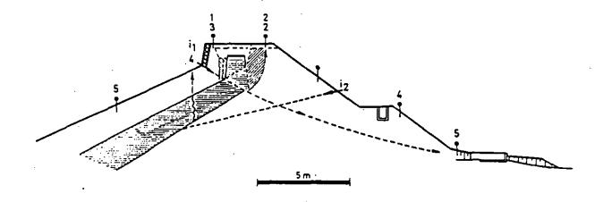
Figure 2: Arrangement of the injection and measuring pipes at the Schwarzenbacher Dam
