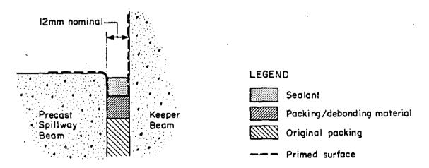
2.3 Precast Beam Joint (Type D)
