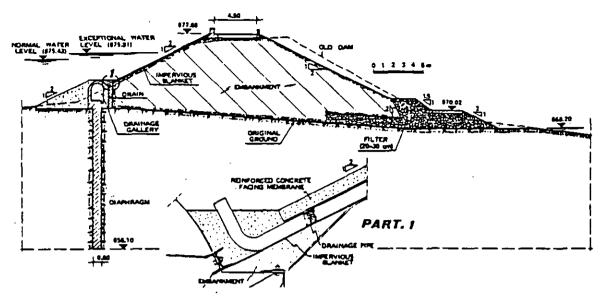
Figure 4: Cross section and particulars of the Coredo main dam
