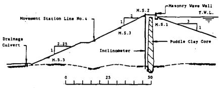
Figure 1: Typical Embankment Section
