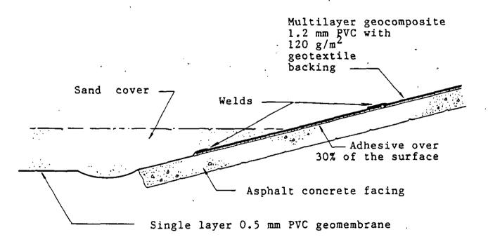
b) Detail of joint at toe of dam.
