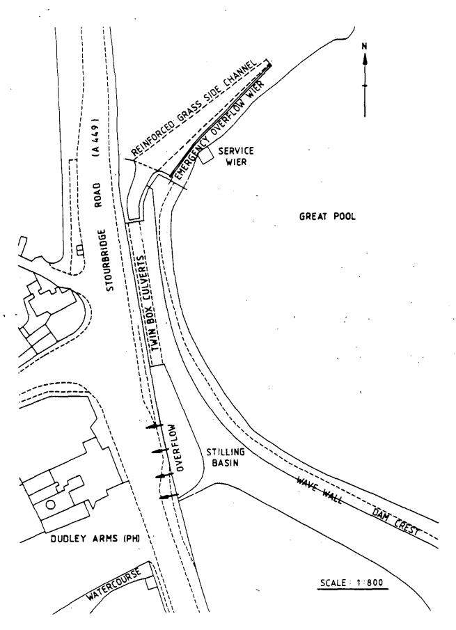
Figure 3: Emergency overflow arrangement.
