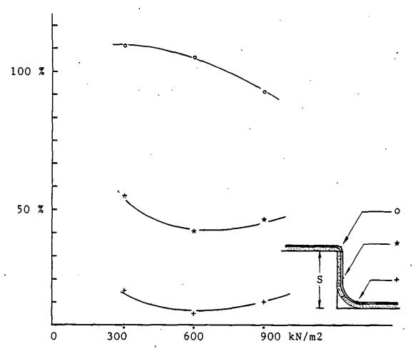
Fig. 3 Water Pressure (kN/m2) - Elongation (%) results of Shear test across a step of S = 35 mm
