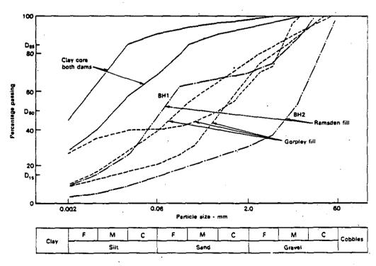
Figure 5: Range of particle size distributions for the clay core and downstream fill from Gorpley and Ramsden dams
