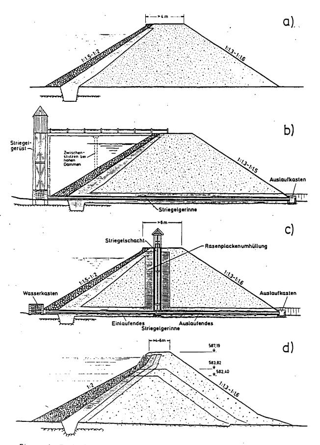
Figure 1: Typical cross sections of mining dams in the Harz mountain area
