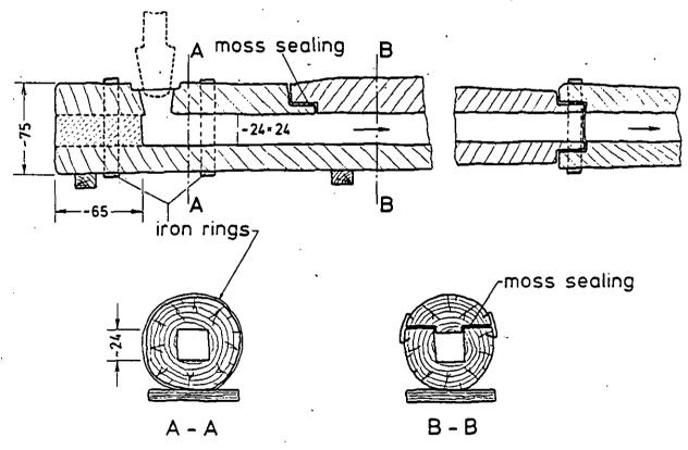
Figure 4: Wooden outlet pipes of the old mining dams
