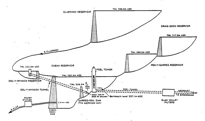
Figure 2: Levels of the Foel Tower and the Elan Valley reservoirs
