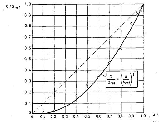
Figure 3: Diagram of the intake capacity depending on degree of ageing (here: stoneware pipe)
