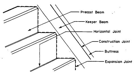
1.3 View of joints at precast beam ends
