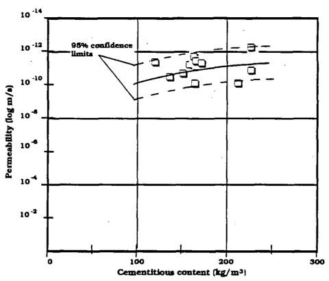
Figure 3: Relationship between in-situ permeability and cementitious content for concretes from conventional dams
