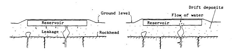
Stage III: Void or fissure penetrates reservoir
