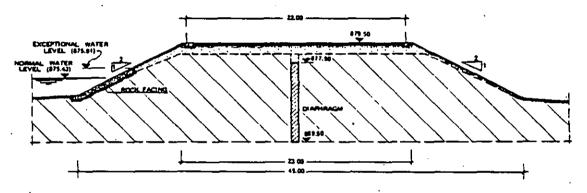
Figure 5: Cross section of the Coredo auxiliary dam
