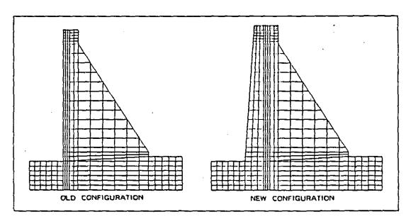
Figure 10: Tres dams: Mesh of the actual and designed solutions
