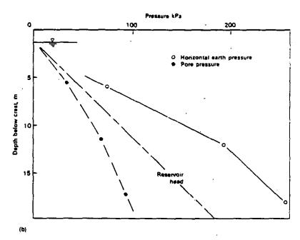
Figure 4: Pressure measurements on centre-line of the clay cores:
