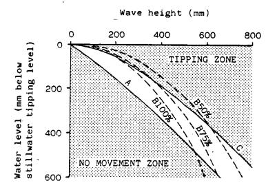
Figure 4: Effect of waves on tipping level of Yeoman Hey gates
