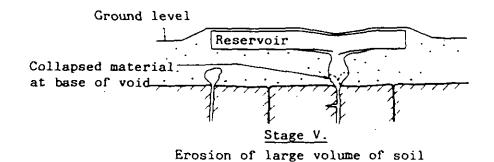
Figure 3: Probable Cause of Subsidence of Reservoirs
