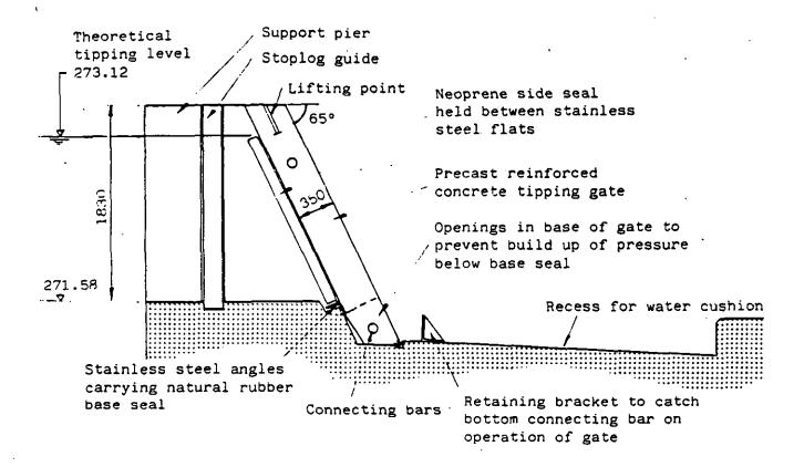
Figure 3: Cross section of Greenfield reservoir tipping gate
