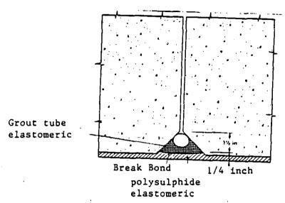
Figure 1. Design for repair of vertical joints in Richard B. Russell dam - Savannah, Georgia
