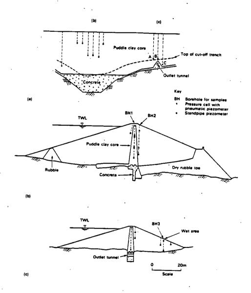
Figure 1: Gorpley dam: (a) longitudinal section; (b) transverse section at centre of dam; (c) transverse section at outlet tunnel
