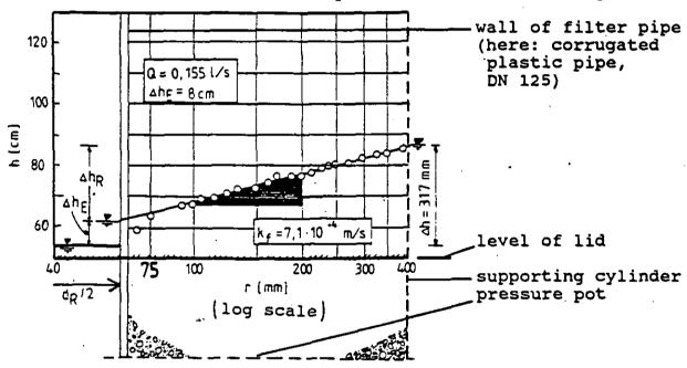
Figure 2: Evaluation of an experiment with the pressure pot
