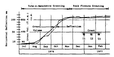
Figure 5: Horizontal Deflection and Grout Volume
