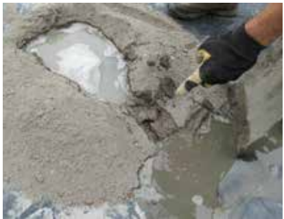
3. As water overflows, the embankment erodes away
