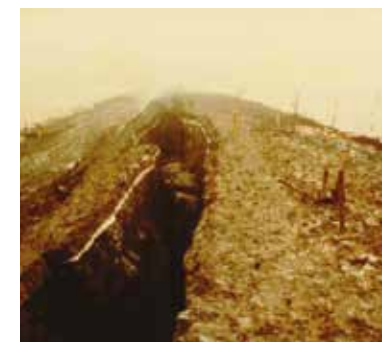
The crack opening at the top of the slip
