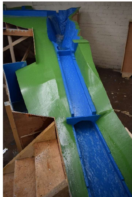
Figure 2 Spillway physical model.
