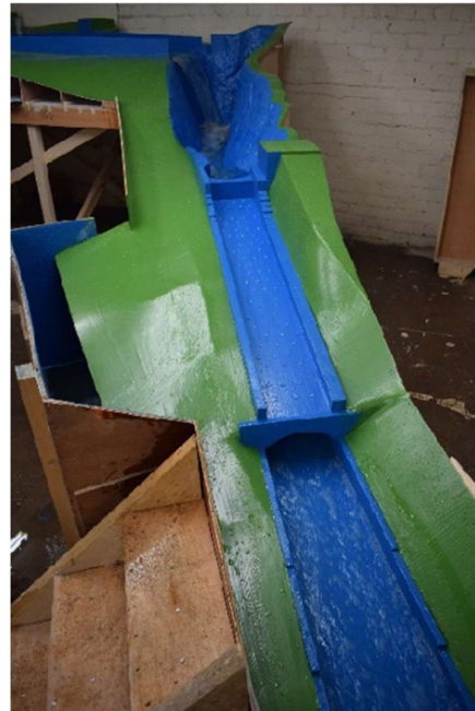
Figure 2 Spillway physical model.
