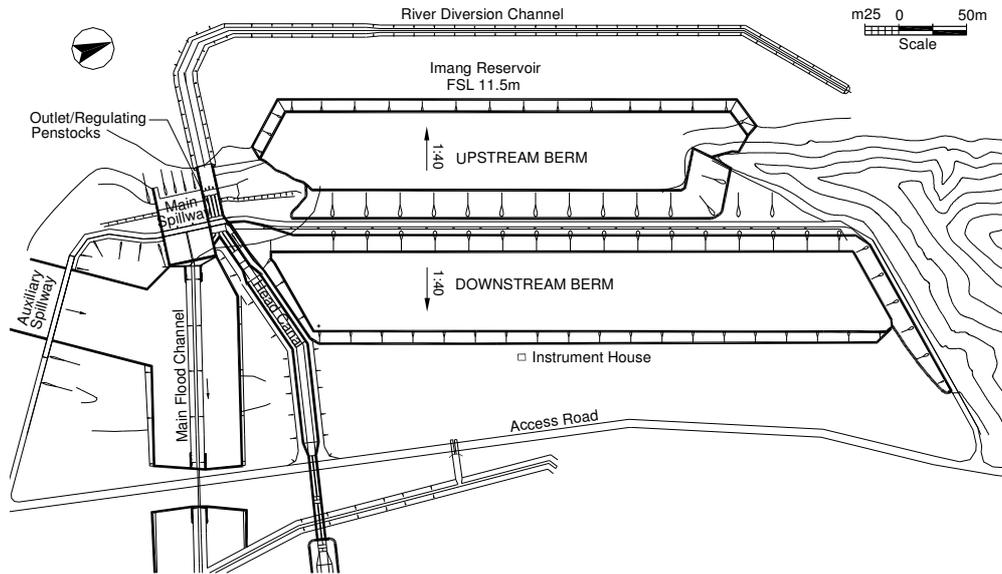
Figure 1 General Arrangement of the Dam and Ancillary Works
