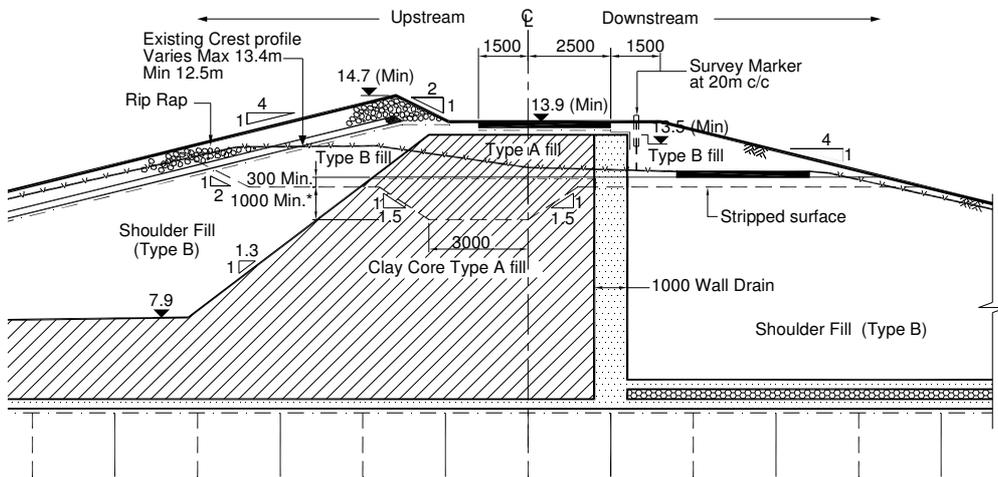
Figure 7 Final Dam Crest Detail
