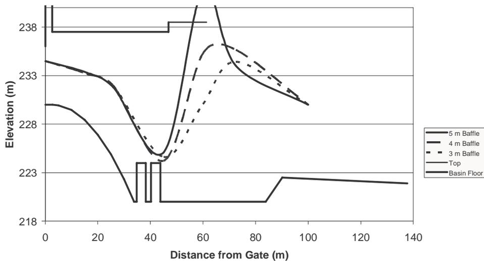
Figure 7: Model Test Results. 75% gate opening and future tailwater level
