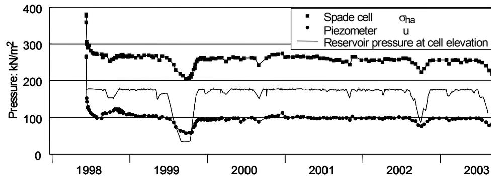
Figure 5: Measurement of horizontal pressure within the rolled clay core of Queen Mother at 17mOD.
