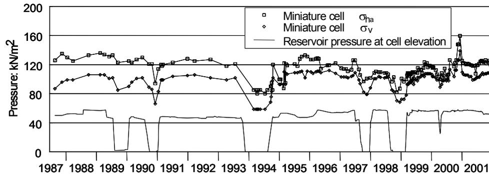
Figure 2: Measurements of vertical and horizontal pressures within the puddle clay core of Staines South at 17mOD.
