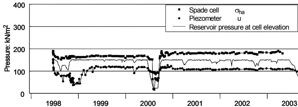
Figure 4: Measurement of horizontal pressure within the rolled clay core of Wraysbury at 15.6mOD.
