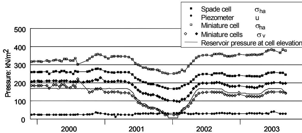
Figure 3: Measurements of vertical and horizontal pressure within the puddle clay core of King George VI at 12mOD.
