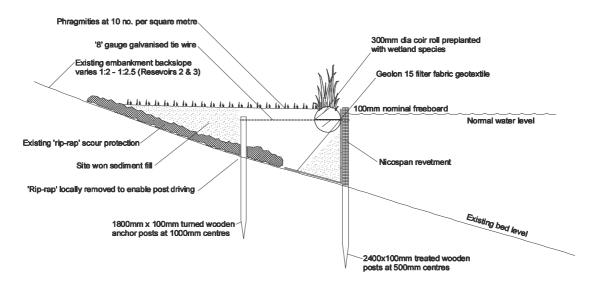
Fig. 6 - Section of "silt" shelf
