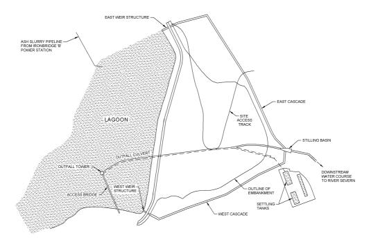
Figure 2: Plan of the embankment at Devils Dingle
