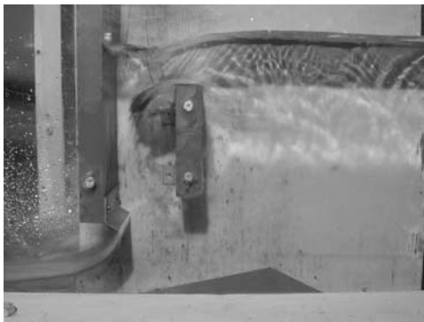
Plate 5 Upstream head still affected by weiring flow over baffle
